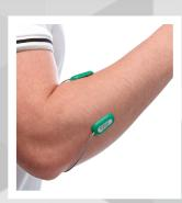
For over 30 years, the Biometrics Electrogoniometer has been the gold standard for dynamic joint angle measurement in fields such as biomechanics, ergonomics, gait analysis and sports science.
