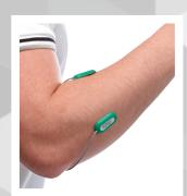
For over 30 years, the Biometrics Electrogoniometer has been the gold standard for dynamic joint angle measurement in fields such as biomechanics, ergonomics, gait analysis and sports science.
