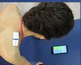
2 channels totally wireless EMG Biofeedback device designed for free use home training. A simple 2 bars graphic is available to guide the exercises. Visual and sound feedback is available.
